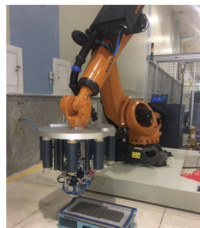
图5 南航8丝束机器人式自动铺丝机 Fig.5 Robot placement machine with 8 tows from NUAA
