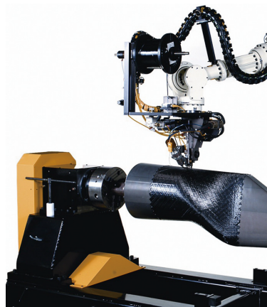
图11 XT系列机器人铺放过程 Fig.11 Fiber placement process of XT series robot
