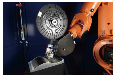
图4 德国弗朗霍夫研究院铺放设备 Fig.4 Robot automatic fiber placement machine from IPT
