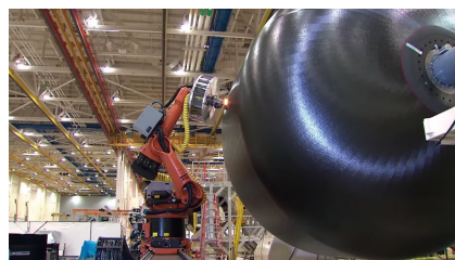
图8 采用红外加热热源的机器人式自动铺丝机 Fig.8 Fiber placement machine with infrared heating source
